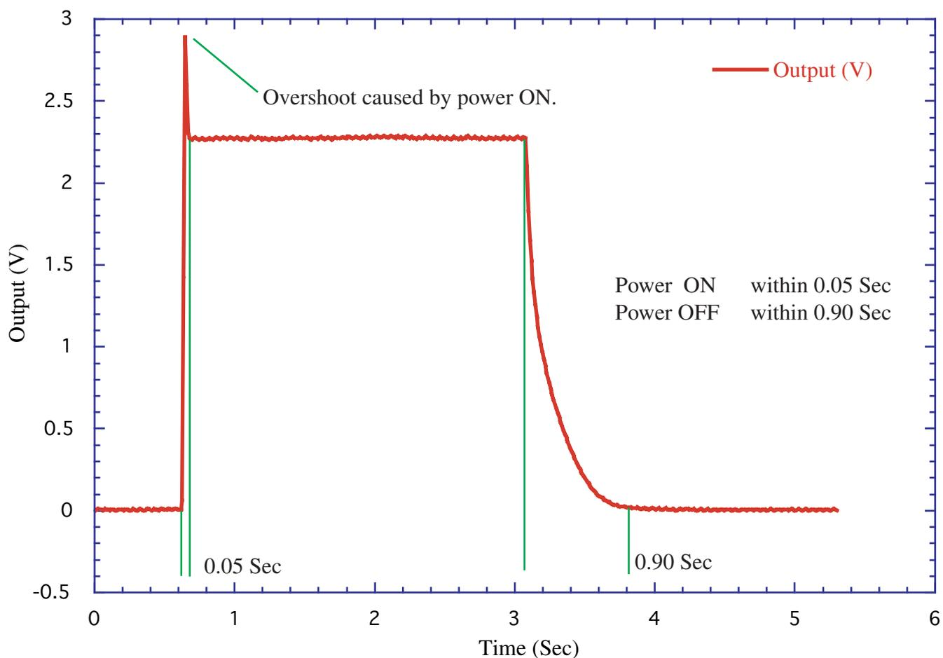
Response time to stable when the sensor powered ON and OFF.
